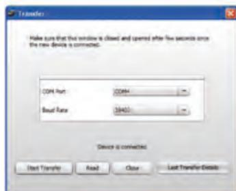
The counter can be programmed straight from a computer using the programming assistant. The counter must be connected to the computer. Click the button "Begin transfer" in the File/Transfer menu to transfer the configuration data to the counter. Click the button "Read" to read out the configuration data on the computer.
