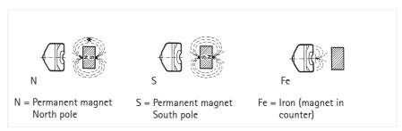
Actuation is effected by a magnetic field. With suitable magnets it is possible to achieve actuating distances of up to 50 mm. The direction of approach of the actuating magnet is not critical. When choosing a counter, it is important to observe the correct polarity of the actuator (see Figure).
