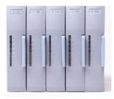
Each Four Loop Controller Module (LCM), is an independent PID controller. Up to a max of eight LCMs can be configured for each Bus Communications Module (BCM). Each LCM contains its own PID processor as well as all input and output connections. Mixed installations of Single Loop and Four Loop LCMs are possible. Each LCM can be removed and replaced (Hot Swapped) whilst the process is running.
