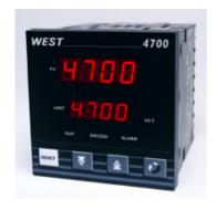
The West 4700 is a safety cut-out, with optional annunciators and alarms. A latched relay cuts process power if safe values are exceeded. A reset is required before continuing.
