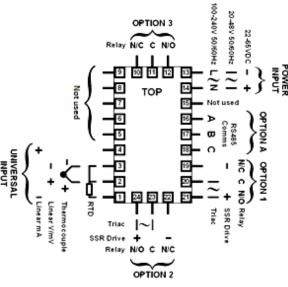
These diagrams show all possible option combinations. The actual connections required depends on the exact model and options fitted.
