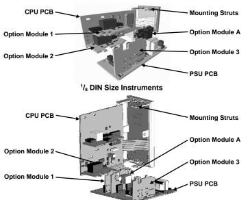
To access modules 1 or A first detach the PSU and CPU boards from the front by lifting first the upper, and then lower mounting struts. Gently separate the boards.
