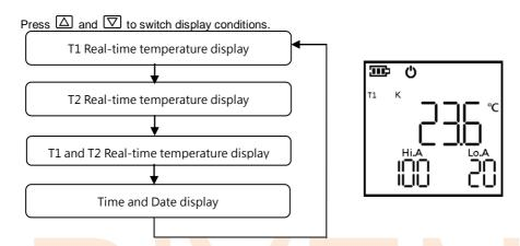
In the testing mode, the display content as below:
