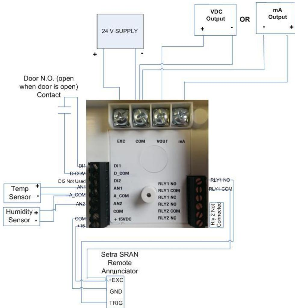
Figure 3-7 Wiring, SRIM2
