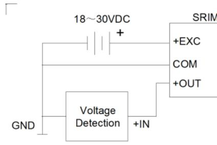
Fig. 3-5 Wiring Diagram SRIM1 and Back of unit
