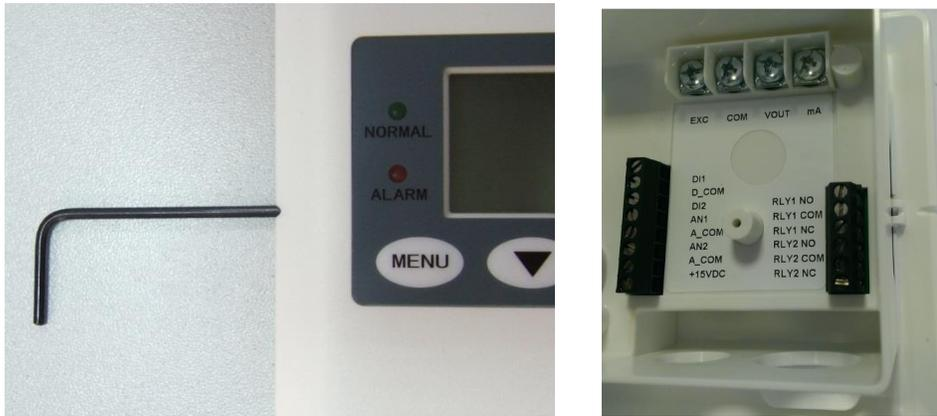
Fig. 3-3 Removing bezel from the base
