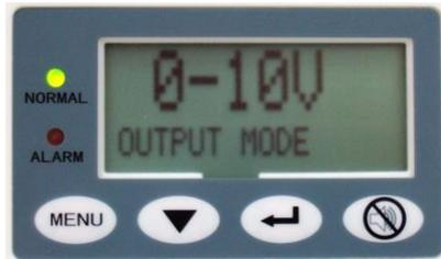
Continue to press the menu key to progress all the way through the menu until you reach the RETURN screen. Press the Enter key to exit out of the menu and return to home screen.
