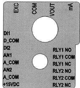
Pull wires through the openings in the bottom of the base. 1/2" conduit or PG9 fitting openings are provided.
