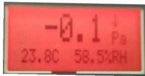
Unit in the alarm state. Red backlight, arrow indicating which parameter and if it above or below alarm limits and audible buzzer if enabled.
