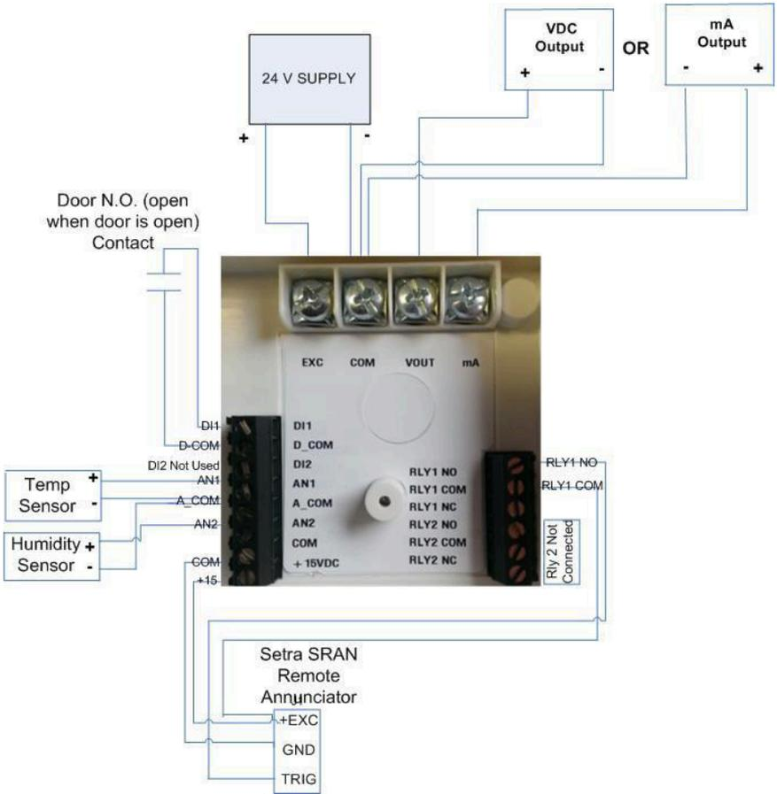
**Fig. 3-7 Wiring, SRIM2**
