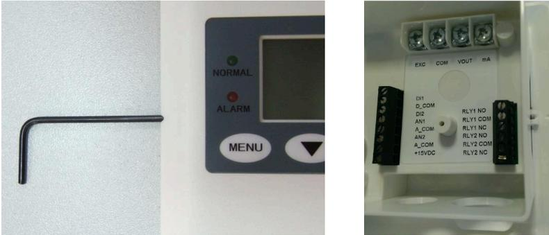
**Fig. 3-3 Removing bezel from the base**
