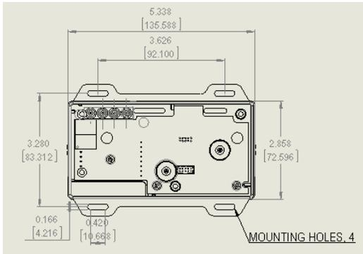
**Fig. 3-1 Wall (flush) mount housing dimensions, front view, SRIM1,2**
