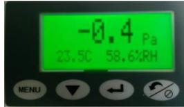
Unit in the normal state, line 1 is the indicated differential pressure and units. Line 2 indicates the temperature and humidity reading, if enabled. The green backlight indicates that the room pressure, the temperature and humidity is within the allowable alarm limits. Note that the alarm will occur if any of the 3 monitored parameters are outside of their respective limits.
