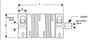
integral 360° clamps which firmly grip the encoder shaft and the input shaft while remaining slip-free to the rated torque of the coupling. NOTE: Shafts may extend beyond the clamp-grip area (G) to the flexure area but they must not butt.
