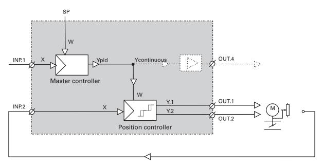
Basically, this controller function is a cascade. A slave controller with three-point stepping behaviour working with position feedback Yp as process value (INP2 or INP3) is added to a continuous controller.
