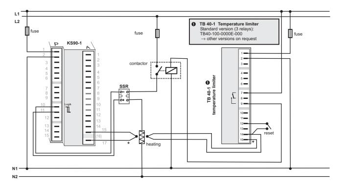
CAUTION: Using a temperature limiter is recommendable in systems where overtemperature implies a fire hazard or other risks.
