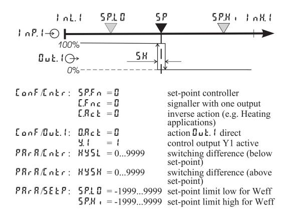
For direct signaller action, the controller action must be changed (LonF / Lotr / LRct = 1)
