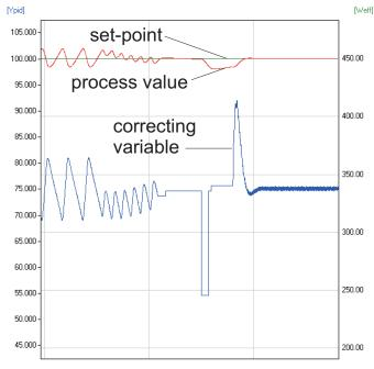
With a *3-point controller*, optimization for the "heating" or "cooling" parameters occurs dependent of the instantaneous condition.
