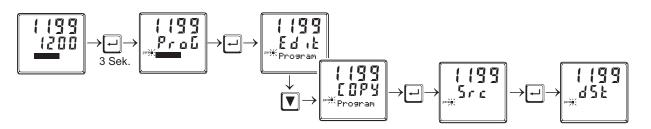
When confirming function COPY with key  $\square$ , the program which shall be copied must be selected (5rc). Subsequently, the target program (d5t) must be adjusted. Press key  $\square$  to start copying.
