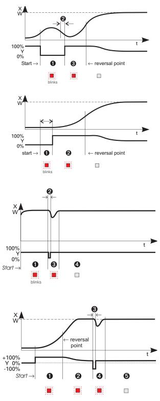
During phase **3**, heating and cooling are done <u>simultaneously</u>!
