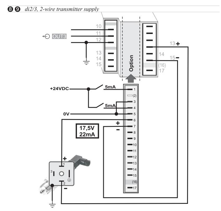
Analog outputs OUT3 or OUT4 and transmitter supply  $U_T$  are connected to different voltage potentials. Therefore, take care not to make an external galvanic connection between OUT3/4 and  $U_T$  with analog outputs!
