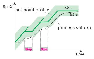
With segment type Step and bandwidth monitoring activated, the control deviation alarm is suppressed, until the process value is in the band again.
