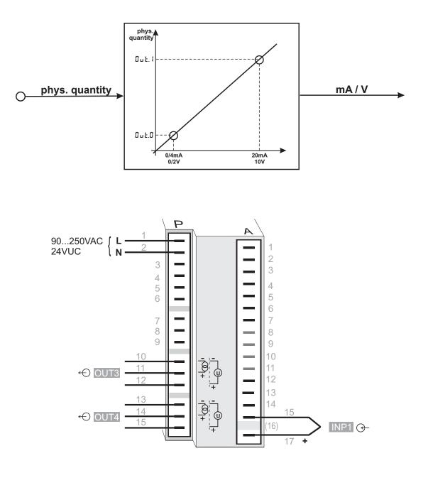
Conf/Out.3/4: OLLYP Dut.3/4 0...20mA continuous 1 = 2  $\Box_{L} E J / \Psi 4...20$ mA continuous = 3 Dut.3/4 0...10V continuous = Ч But.3/4 2...10V continuous = scaling **Dut.3**/4 8.4u8 -1999...9999 = for 0/4mA or 0/2Vscaling **Dut.3**/4 But.1 -1999...9999 = for 20mA or 10V signal source for **Dut.3**/**Y** is 0.5rc =3 the process value
