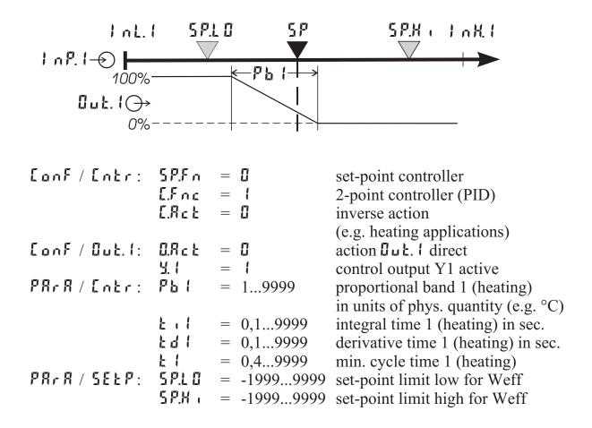
For direct action, the controller action must be changed (LonF / Lotr / L.Rct = 1).
