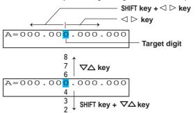
When you press the  $\ensuremath{\vartriangleleft}$  key, the change is applied and the next setup item is displayed.
