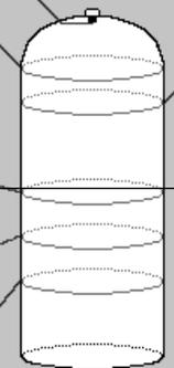
**Sensor Height:** Distance from the bottom of the tank to the bottom of the transducer.
