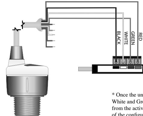
\* Once the unit has been configured, the White and Green wires must be isolated from the active power to prevent a shorting of the configuration circuit.
