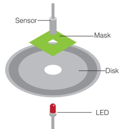
**Figure 7:** Traditional Optical Encoder Engine
