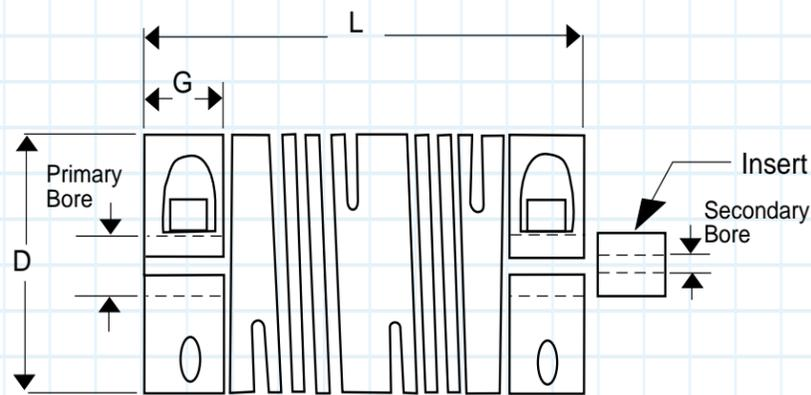
Shafts may extend beyond the clamp-grip-area to within the flexure area, but must not butt.
