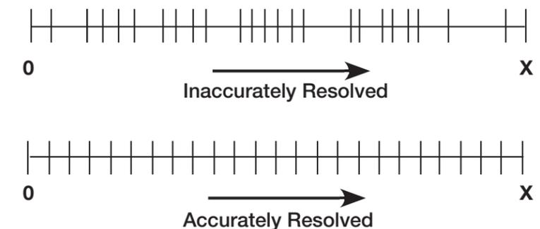
**Figure 1:** Resolution and Accuracy
