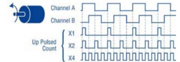
**Figure 2:** A quadrature encoder generates two pulse streams that are 90° out of phase with one another. As a result, the system can determine directionality by monitoring which channel leads in phase. Triggering off of the leading and or trailing edges of the pulses can increase resolution by up to four times.
