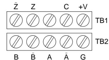
Screw terminals with pressure plates that accept #14 AWG to #22 AWG.
