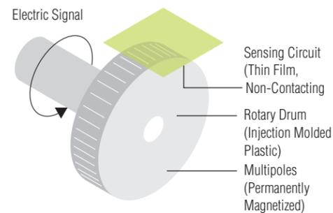
**Figure 9:** Incremental Magnetic Technology
