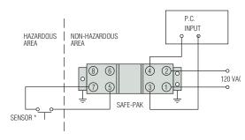
Programmable SAFE-PAK, P/N 54825, providing simple on-off functions for hazardous location, and interfacing with TTL or AC logic input of programmable controller. \*Temperature, pressure, position, flow or level.
